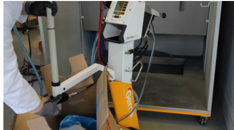
Step 2: Raise the suction tube
