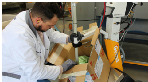
Step 6: Lower the suction tube in the new colour
