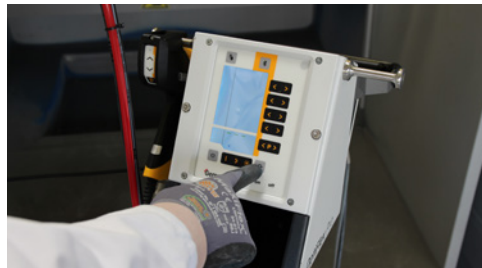
Step 4: Start the cleaning process
