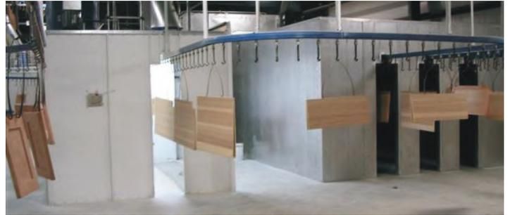
With a low-temperature oven attached to an enclosed finishing booth via a vestibule, painted products can quickly be stacked on carts and rolled into the low-temperature oven. There are substantial upfront and operational cost savings from not adding an air make-up unit (AMU) to an enclosed finishing booth. Having a low-temperature oven attached to a booth also allows products to remain in the same environment during painting and curing, which leads to a better quality finish.
