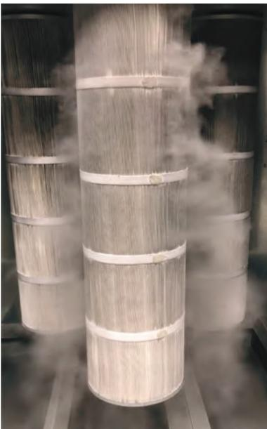
powder, a magnetic gauge on the side of GFS powder coating booths monitors the booth's pressure drop. Once a preset pressure drop is reached, the filters pulse, allowing powder to fall into the fluidized beds or drawers or onto the floor of the booth.
