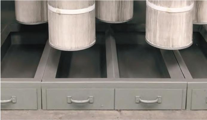
Similar to fluidized beds, drawers collect wasted powder so that it can be discarded or reused. Removable drawers are located beneath the filters. When the filters pulse, the powder from the filters drops into the drawers.
